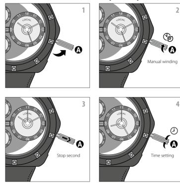
Automatic caliber 🚯: Manual winding and time setting
